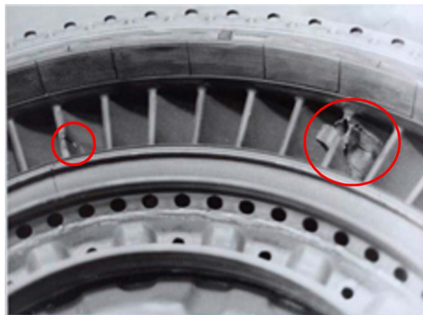
Fig. 2 Turbine stator vanes burn
